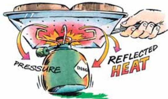
When heated, the liquid gas inside the canister will start to boil which leads to an increase in pressure inside the canister. Exposure to temperatures higher than 50° Celsius will lead to dangerous pressures that may rupture the canister. If there is any source of ignition, the escaping gas will ignite creating a large explosion.
