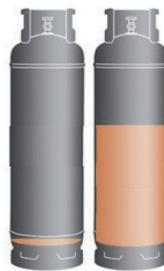
If demand is more than 50 MJ per hour the auto change over will draw LPG from the second cylinder to make up the required gas flow.
